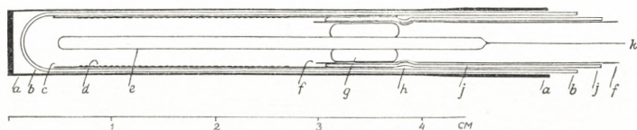
Fig. 1. Small boron chamber. a , outer brass tube; b , soft glass tube providing insulation between a (earthed) and c ; c , the high tension (100 Volt) electrode with the boron lining d ; e , collecting electrode, connected to the amplifier by the thin wire k ; f , grounded shield, insulated from c by the glass tube j , which is punched ( h ) to keep the insulating glass bead g in position.
